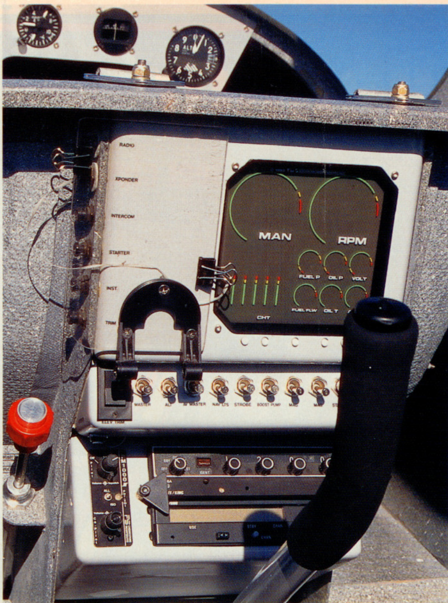
Electronic engine instrumentation and basic avionics are mounted in front of the Giles 202's backseat stick (above); the flight instruments are located in the front cockpit. Although G-limit testing is still in progress, the composite airplane's roll rate is about 400 degrees per second.
