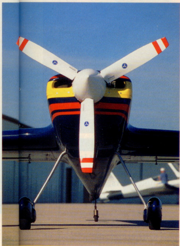
In this installation, a modified Lycoming AEIO-360 turns the 202's three-blade composite propeller.
